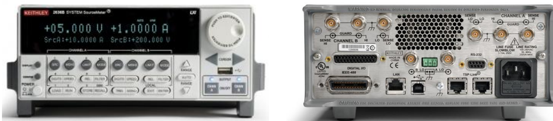
Figure 6. Front (left) and back (right) views of the Keithley 2636B 2-channel low-current sourcemeter.
